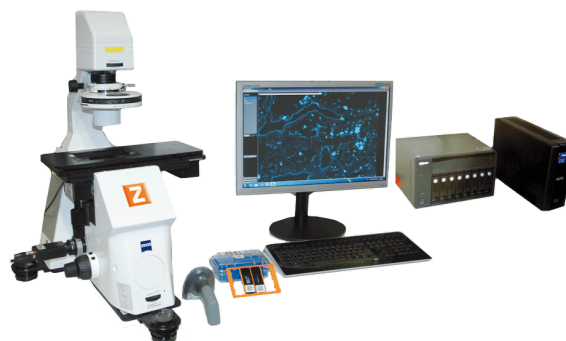
Figure 2. The ChipCytometry workflow uses the ZellScannerONE, an all-in-one instrument that combines iterative rounds of immunofluorescence imaging with advanced image analysis software for cell phenotyping and quantification.
